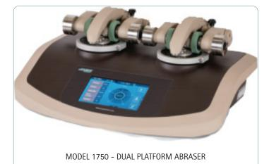
"Taber Test" delivers reliable data in minutes. Used to evaluate a material's resistance to wear, a flat specimen is mounted to a turntable platform that rotates on a vertical axis. As the turntable rotates, contact of the specimen against the sliding rotation of two abrading wheels cause wear while a vacuum system removes loose wear debris during the test. The resulting abrasion marks form a pattern of crossed arcs in a circular band that cover an area approximately 30 cm<sup>2</sup>.
